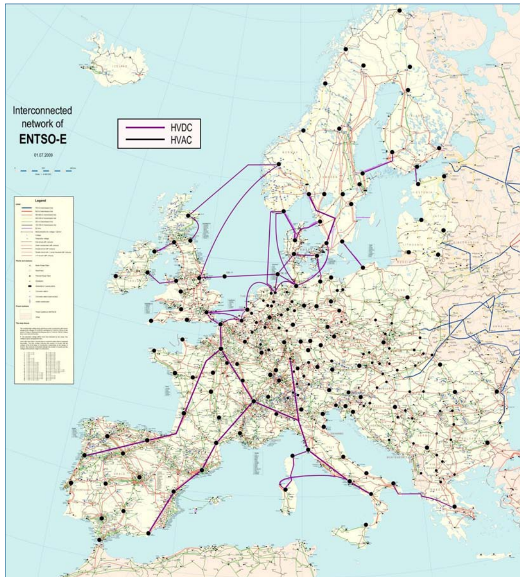
Figure 17: Map of the high-voltage network of Europe with the proposed HVDC grid (Status 2030). Source: ENTSO-E, energy-nautics
