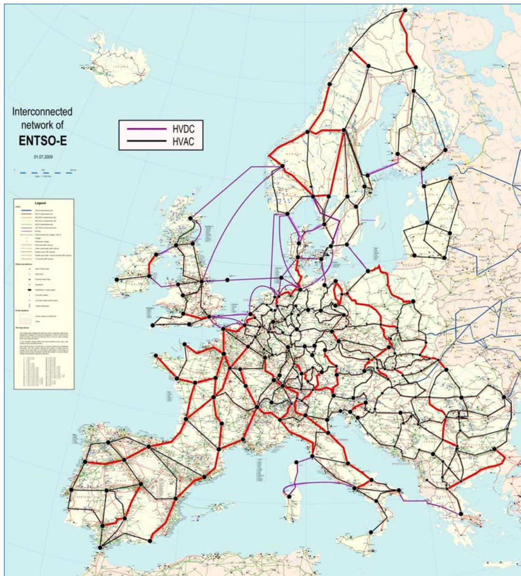
Figure 16: Map of the high-voltage network of Europe (Status 2030) with the overlaying simplification marking upgrades of the European power system. Source: Reproduced with permission of ENTSO-E, energynautics
