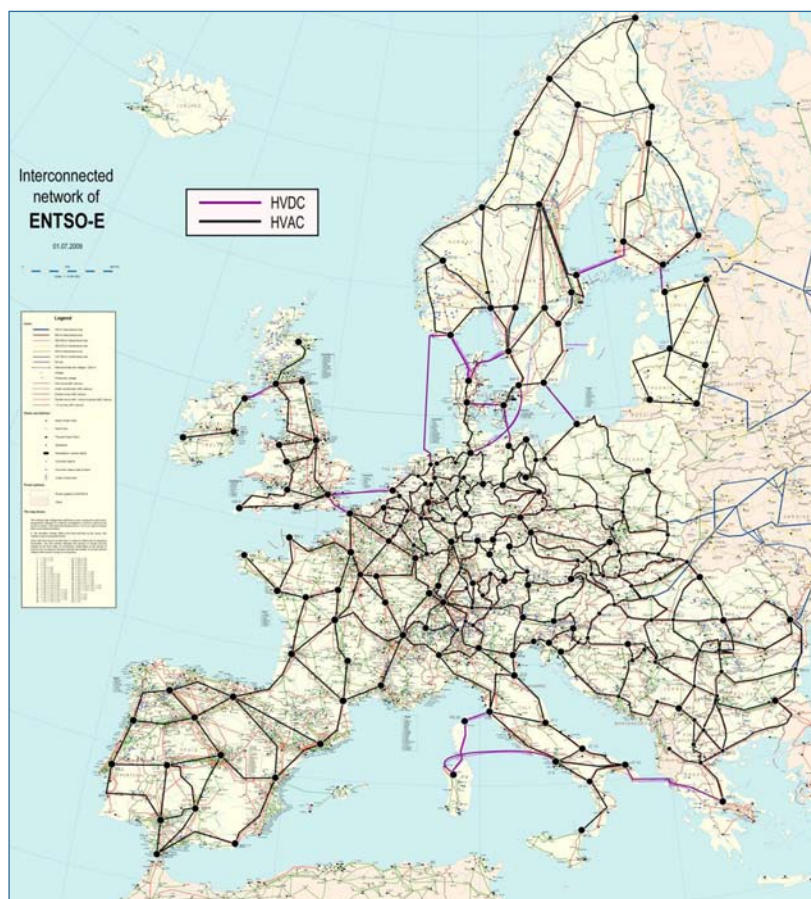
Figure 3: Map showing energynautics ' model of the high-voltage network of Europe (Status 2010), based on 224 grid-connected nodes. Source: Reproduced with permission of ENTSO-E by energynautics
