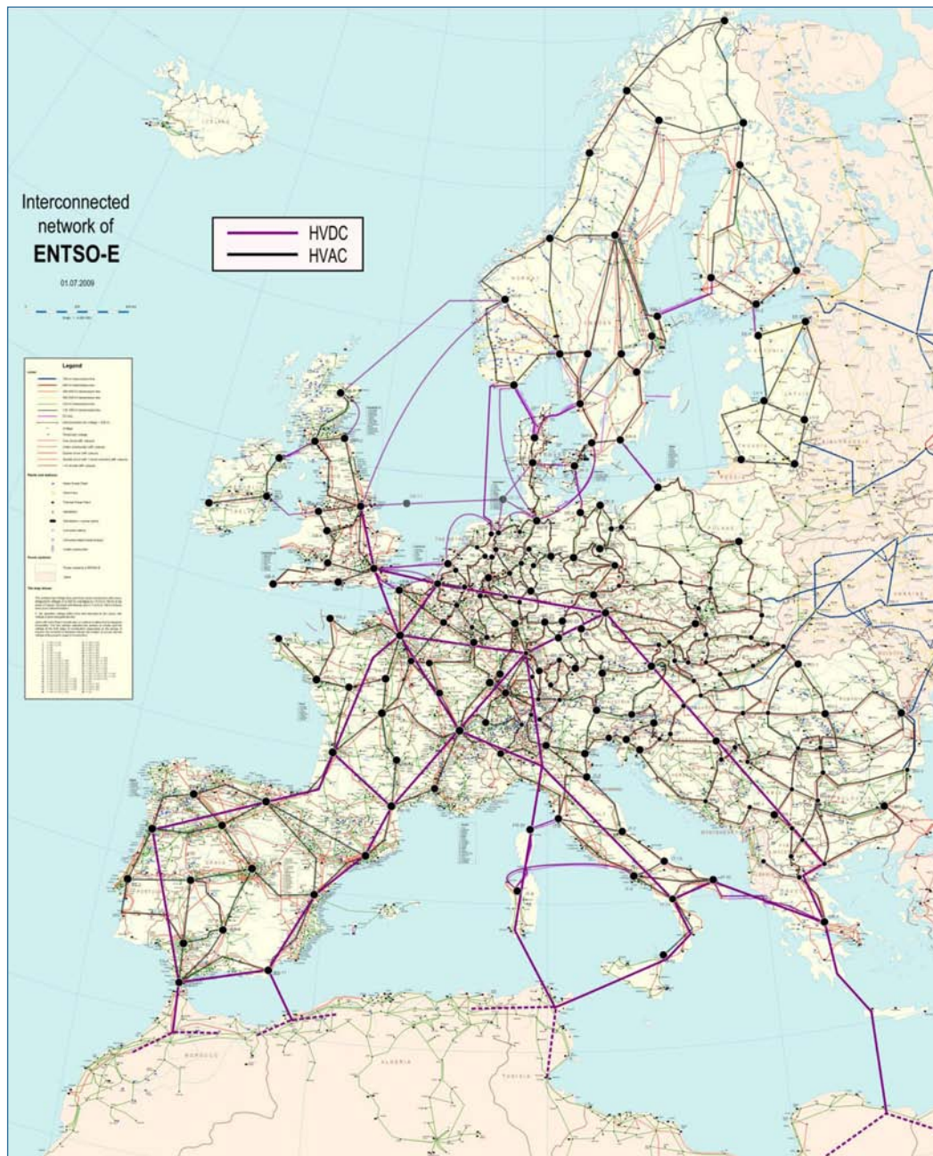
Figure 21: Map showing energynautics' model of the high-voltage network of Europe (Status 2050), based on 224 grid-connected nodes. Source: Reproduced with permission of ENTSO-E by energynautics.
